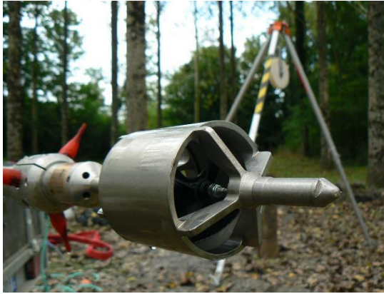
Micromoulinet GEOVISTA (diam 75 mm)
